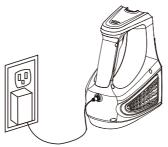
2. The LED indicators will show the progress of the charge. While the vacuum is being charged, the LED indicators will be flashing blue alternately. Once fully charged, the LED indicators will show static blue lights. The battery requires approximately 4~5 hours of charging to regain full capacity.
