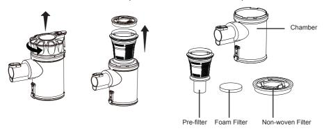
3. Brush loose debris from filters then rinse with warm water. Rinse and gently squeeze dry the foam filter. Set both filters aside and allow to air dry for 24 hours.
