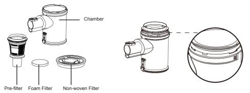
5. Place the filters back onto the pre-filter. With the dust cup release button facing away from the wand connection on the dust cup, lock the top into place by rotating clockwise.
