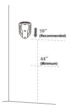
4. To store, hang the hand vacuum on the wall mount. Align the slot on the bottom of the hand vacuum with the protrusion on the wall mount as shown in the picture below.
