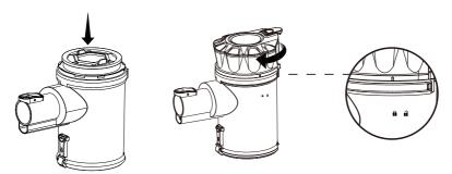
6. To reassemble the dust cup to the hand vacuum, align the slot in the dust cup to the hand vacuum. Once aligned, press down on the dust cup release button until you hear a click.
