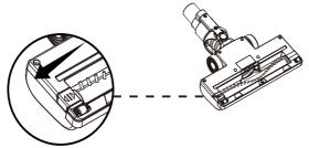
3. Simply lift the brush roll out of the nozzle housing. Clean off debris and anything wrapped around the brush roll. Use a pair of scissors to remove threads, etc.
