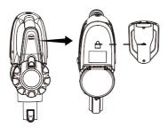
5. Insert the 2-in-1 combination tool into the right slot on top of the wall mounting bracket for convenient storage. Insert the crevice tool into the left slot.
