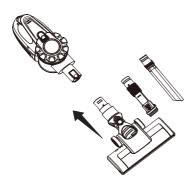
3. When finished cleaning, turn the vacuum cleaner off and press the wand release button to remove the motorized nozzle or accessory tools.
