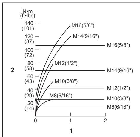
► 1. Fastening time (second) 2. Fastening torque
