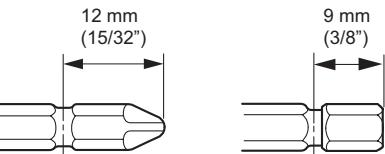
Use only the driver bit/socket bit shown in the figure. Do not use any other driver bit/socket bit.
