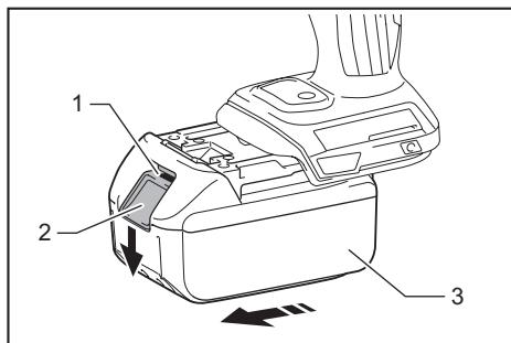
To remove the battery cartridge, slide it from the tool while sliding the button on the front of the cartridge.
