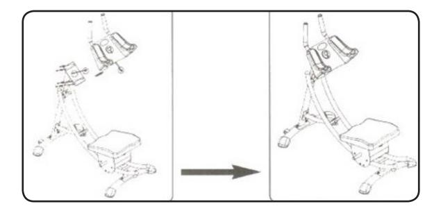
**Step 5:** Connect the counter wires in 2 locations as shown. Install the wire protection covers to cover the wire connections.
