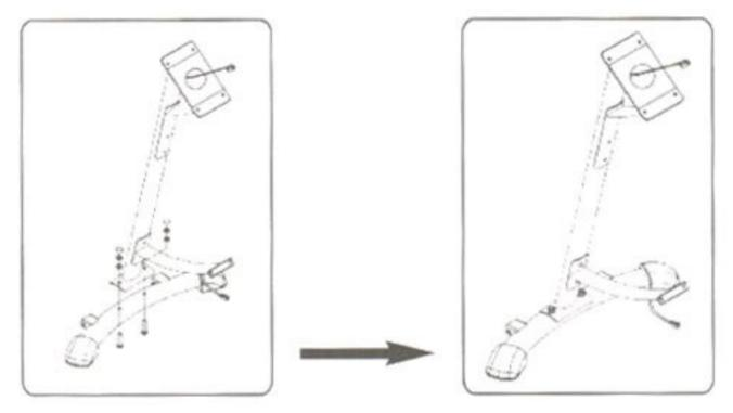
**Step 3:** Attach the front post to the curved track. The front post is attached to the track in two locations as shown using the 2 pre-attached Allen head screws for each location. Finger tighten only.
