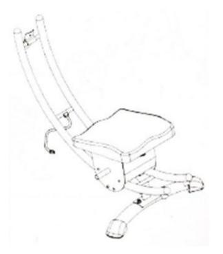
**Step 2:** Attach the front foot (with wheels) to the front post using the 2 pre-attached bolts. Finger tighten only.
