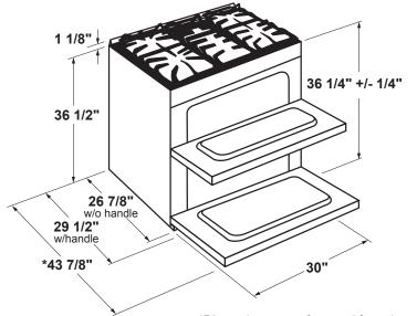
\*Dimensions are referenced from the point at the back of the range that will contact the rear wall first.
