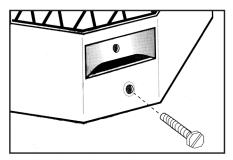
1. Insert one screw into the lower hole located in each mitered corner of the chimney cover band. (Just start the screw into the hole a few turns, until all four screws are started.)
