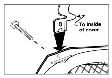
1. Slip the leg up through the lance inside each corner of the band until the hole in the leg is aligned with the hole in the lanced band. Insert the mounting screw (use the same four screws enclosed with cover) through the hole in the leg and into the hole in the lance. Tighten the screws just enough to hold the legs into the lanced slots on each corner of the cover. **Do not tighten fully at this time.**
