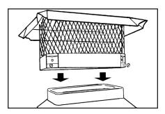
2. Place the chimney cover on the flue tile and align the base with the flue liner. Partially tighten each of the four screws until they are snug to the tile. Then tighten each of the four screws firmly to the tile.
