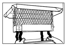
2. Insert two (2) legs into the liner no more than 1". By exerting pressure as shown, force the other legs inside the liner. Push cover straight down into the chimney liner as far as possible. Tighten the screws on all four (4) legs until the cover is held firmly into the flue tile.
