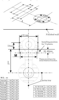
Drawing for distance of installing holes
