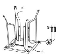
Place table top frame (J) on the ground, then screw table legs (K) to it. Please do not tight any screws to the end at this step.
