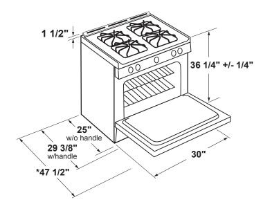
\*Dimensions are referenced from the point at the back of the range that will contact the rear wall first.
