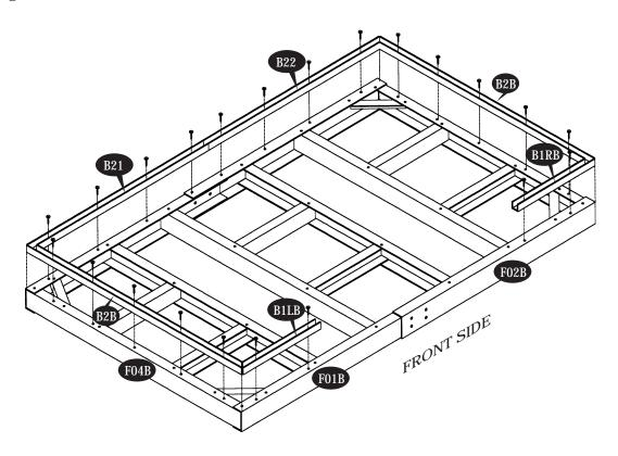
7a. After completing the assembly of shed place exterior grade CDX  $3/4"\ (19mm)$  plywood inside the foundation. See fig.
