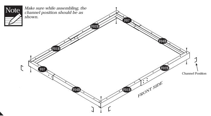
4. Fix the L-angle (F03) to the channel at all the four corners to make a perfect frame. See Fig.
