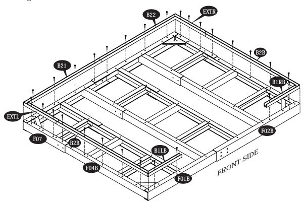
8a. After completing the assembly of shed place exterior grade CDX  $3/4\ensuremath{"}$  (19mm) plywood inside the foundation. See fig.
