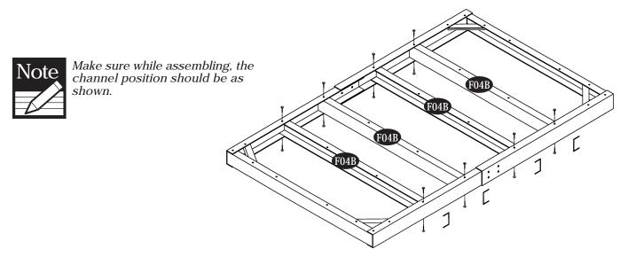
$5. \ \mbox{Fix}$  the channel (F05B) into the frame with screws as shown. See Fig.
