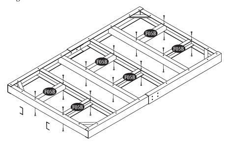
$\ensuremath{\mathbf{6}}.$  Assemble the U-Channel bases on top of the foundation as shown in Figure.
