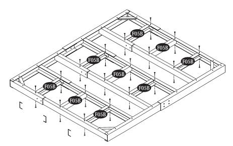
$7. \ \mbox{Assemble}$  the U-Channel bases on top of the foundation as shown in Figure.
