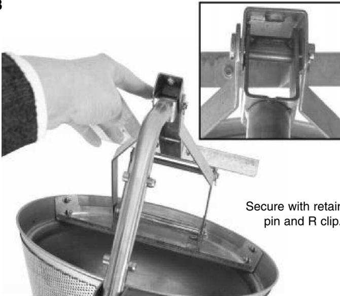
Secure with retaining pin and R clip.
