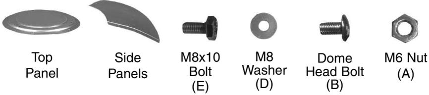
Remove any protective layer and loosely screw parasol side panels together overlapping as shown with 18 dome head bolts and nuts (B,A), fix the top panel to the top of assembled side panels. Tighten all nuts. Fix assembled parasol onto top of Parabolic Reflector Bracket using 3 M8x10 Bolts (E) and M8 washers (D).
