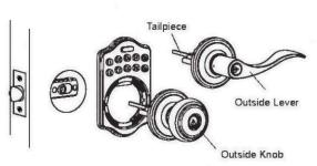
b. Pass the IC wire over the latch to the interior side of door. Do NOT pinch wire.
