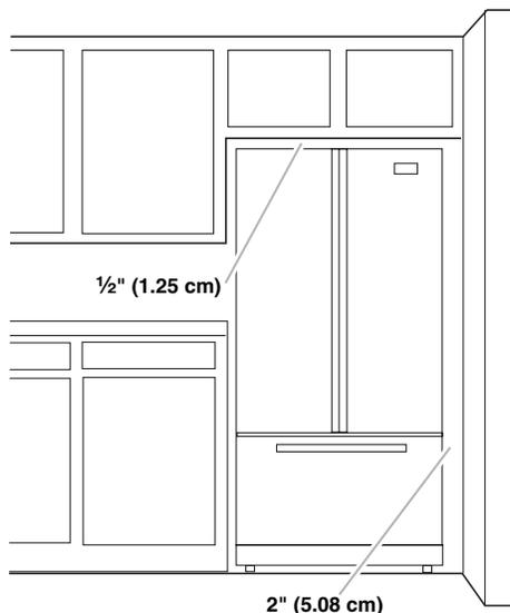
To ensure proper ventilation for your refrigerator, allow for a  $\frac{1}{2}$ " (1.25 cm) space on each side and at the top. Allow for 1" (2.54 cm) of space behind the refrigerator. If your refrigerator has an ice maker, make sure you leave some extra space at the back for the water line connections.
