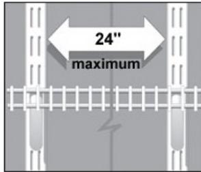
Standards are available in several lengths, depending on the number of shelves you want and the spacing between the shelves. The closer the Standards are placed together, the stronger the installation. Standards should be spaced no more than 24" apart, and no more than 4" from the end of the shelf.
