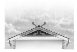
To calculate the minimum amount of total ventilation required, use either the 1/300 or 1/150 ratio. On the inside, the actual calculations have been made for your convenience. Use the 1/300 ratio if you have proper distribution of soffit and ridge vents or if a vapor retarder is present. Use the 1/150 ratio if proper distribution of soffit and ridge vents cannot be achieved and a vapor retarder is not present.
