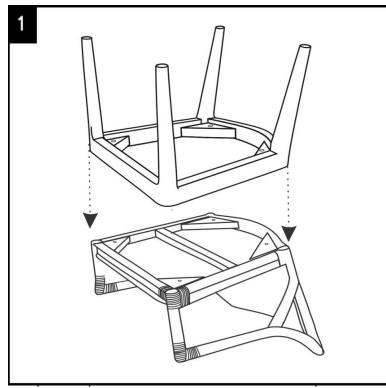
Assembly part A and B with Nuts and tighten with L key
