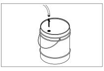
**STEP 1:** Remove detergent suction tube from container and insert into one gallon of fresh water. Slide nozzle forward for low pressure or to connect black detergent nozzle. Pull trigger on spray gun and siphon water for one minute.
