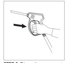
**STEP 5:** Trigger the spray gun to eliminate trapped air then wait for a steady flow of water to emerge from the spray nozzle.
