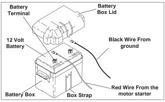
**STEP 8:** Place battery in battery box. Use a standard 12 volt battery.
