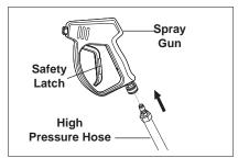
**STEP 1:** Attach the high pressure hose to the spray gun using teflon tape on hose threads.
