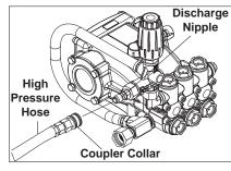
**STEP 5:** Connect the high pressure hose to the discharge nipple. Push coupler collar forward until secure.
