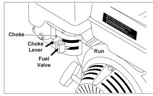
**STEP 7:** Move the choke lever to the "Choke" position (on a warm engine, leave the choke lever in the run position).
