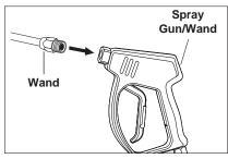
**STEP 2:** Attach wand to spray gun using teflon tape on wand threads.
