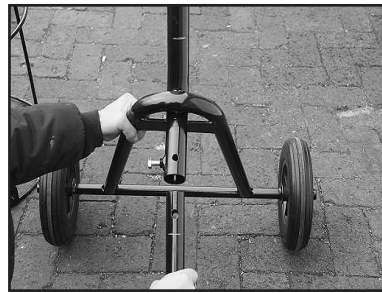
Step 3 Insert Draw Bar into Main Frame.
