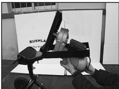
Step 9 Install Gear Motor with the Nuts and Washers. They were removed before
