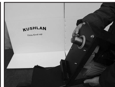
Step 9 Install Gear Motor with the Nuts and Washers. They were removed before
