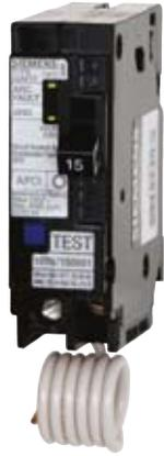
Siemens Combination Type AFCI trip indicators provide a valuable analysis tool to help electricians pinpoint the type of trip. These indicators are in the form of LEDs that appear near the handle of the breaker. The LED indications will appear for 5 seconds each time the AFCI is turned "ON" up to 30 days after the last trip.
