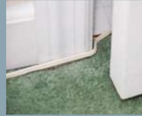
Damaged power supply cord (Example: door continually "pinches" cord)
