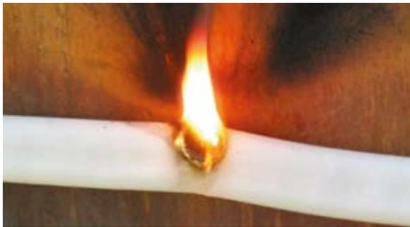
The heating of surrounding materials creates a carbon remnant that acts as a high impedance conductor. As the carbon path extends, the by-products of the arc increase the available fuel source, magnifying the likelihood of a fire.
