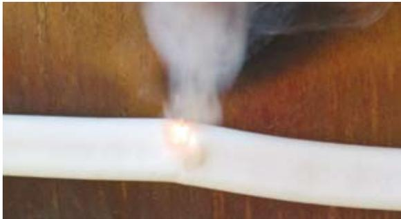
Arcing faults, which can and generally do go undetected by traditional circuit protection means, can reach extraordinarily high temperatures — upwards of 9,000 degrees Fahrenheit.
