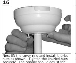
Next lift the cover ring and install knurled nuts as shown. Tighten the knurled nuts securely. The canopy should adjust for any irregularity in the ceiling or Outlet box.
