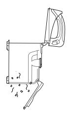
1 Empty dust cup when debris reaches MAX fill line. Remove by pulling up on latches on dust cup handle.
