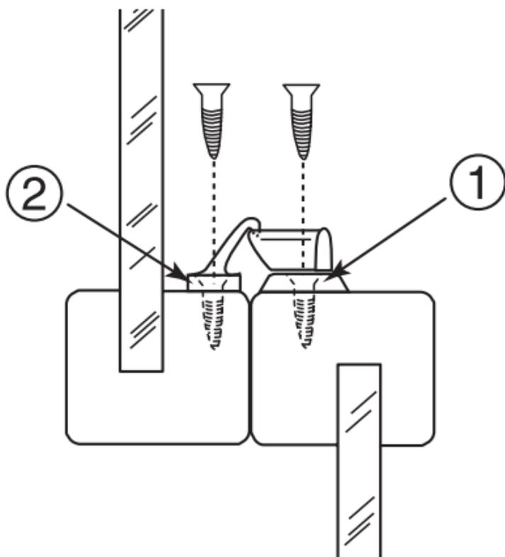
Mount latch (1) in existing holes or mark new location and pre-drill  $3/32''$  new holes. Install and set to locked position. Align keeper (2) under cam, pre-drill holes and install.
