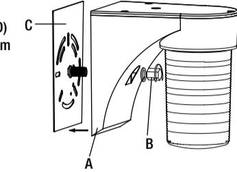
**Installation****2 Installing the mounting bracket assembly**
