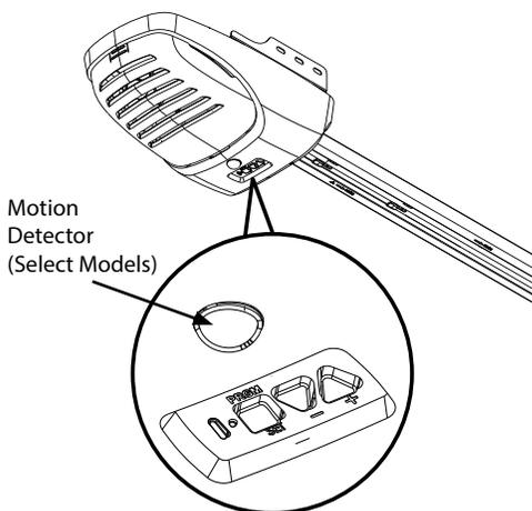
**NOTE:** The 3 programming buttons are for programming ONLY. These buttons CANNOT be used to operate the opener once the required programming section has been successfully completed.
