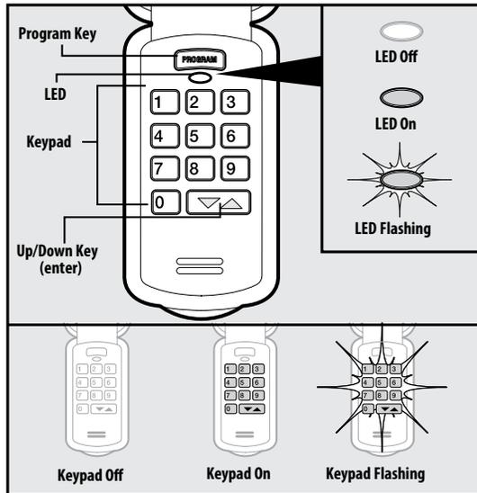
Activate keypad by opening battery compartment and pull protective tab. Reinstall compartment door to begin programming.
