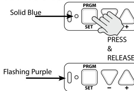
**NOTE:** *The openers LEARN LED will time out in 30 seconds. Programming must be completed within 30 seconds.*
