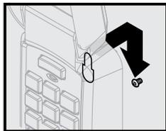
5. Mark and drill a 3/32" pilot hole for the bottom screw and secure keypad to the wall. (Do not over-tighten).
