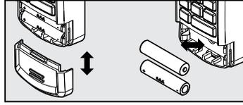
1. Remove battery cover and batteries.
