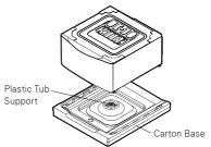
If you must lay the washer down to remove the base packaging materials, always protect the side of the washer and lay it carefully on its side. DO NOT lay the washer on its front or back.
