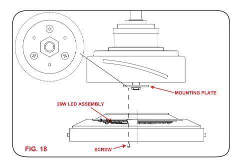
Step 3. After you installed the 26W LED assembly into the fan motor assembly mounting plate, firmly snap the wire connection plugs together. (Fig.19)
