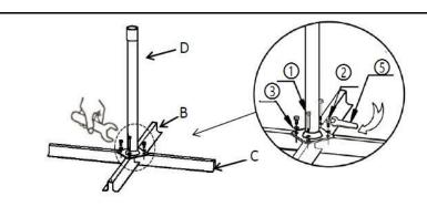
Attach the Base Pole(D) and Steel Cross Base(B) using Washers(E) andBolts(F) with Wrench(J) and Base Pole (D) to Steel Cross Base(C) usingWashers(E) and Bolts(G) with Wrench(J).
