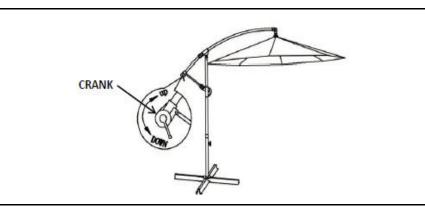
Open the Canopy Sunshade by rotating the Crank clockwise. To close, rotate the Crank counterclockwise.
