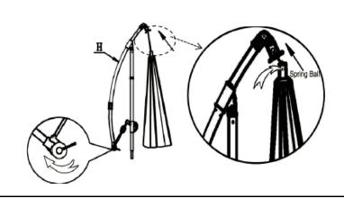
Reel-in the Canopy Sunshade by rotating the Crank clockwise until it touchesthe Frame. Press the Spring Ball on the Canopy and insert the Canopy into the Frame. Rotate the Canopy until the Spring Ball snaps into the mounting position of Frame.
