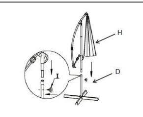
Insert the pole of the Canopy Sunshade(H) into the Base Pole(D) aligning themounting positions of (H) and (D). Screw in by hand the Screw With Acrylic Cap(I) in the mounting positions of (H) and (D) to ensure that the pole is tightly secured to the base. Your Canopy Sunshade is fully assembled. Caution: It is recommended that weights ( $\geq$  45kg), be placed at the base toachieve stability during use of the Canopy Sunshade.
