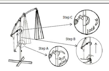
To use the Canopy Sunshade, you need to apply a 3 step process. These are :Step A - First push the lever of the Hand Grip upwards to unlock the CurvedSupport Pole. Step B - Then slide the Hand Grip upwards along the pole about one meterabove the ground. Step C - To lock, pull down the lever of the Hand Grip to lock onto the CurvedSupport Pole into position.
