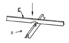
Put the Downward Steel Cross Base(C) on Upward Steel Cross Base(B) and intersect at the notches.
