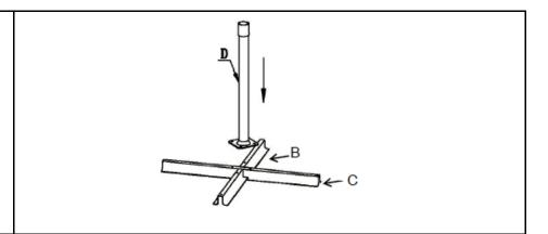
Align the mounting positions of the Base Pole(D) with Upward Steel Cross Base(B) and Downward Steel Cross Base(C).
