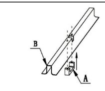
Place the Cross Base Stabilizer(A) under the Upward Steel Cross Base(B) and align the mounting positions of each.
