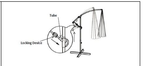
Push the Bend Pole upwards until it is aligned to the Tube. Push down the Locking Device until it covers the Tube. This action locks the Curved Support Pole in position.
