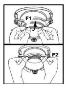
F. Hold the three parts in place while attaching the Retainer Ring (F1) by pulling it apart and having it snap within the groove of the sink flange (F2).
