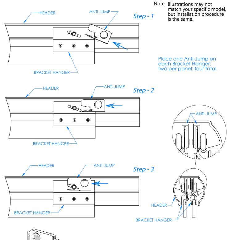
If the Anti-Jump does not stay in the place or -if it is difficult to insert, snap off the "roller side leg" leaving one remaining leg.
