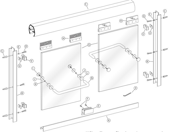
\*\*If installing on a fiberglass unit you may need to snip outside corner to match corners on wall jambs and tub tracks to match radius on fiberglass unit\*\* Measure the wall-to-wall opening at the center of the tub rim. Cut the tub track [A] 1/16" short of this dimension. An inexpensive miter box available at your local hardware store will help you get clean square cuts.
