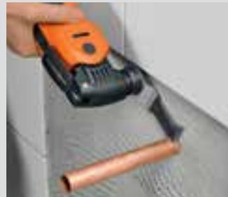
Sawing flush with the wall when space is extremely tight.
