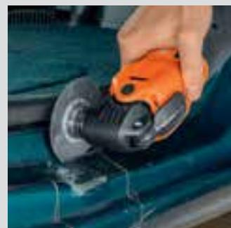
Distortion-free sawing, clean cut edges, thin cutting line – great for car body work.
