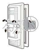
To replace the Door-in-Door case, line up the tabs on the Door-In-Door case with the slots on the door and push down until it snaps into place.
