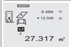
The tool saves measurements and the results of calculations continuously while in operation. A total of up to 30 values, including graphic symbols, are saved in this way. The complete set of information displayed is saved in the following situations:
