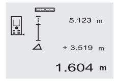
The tool can be used to indicate given distances, e.g. when setting out and marking the position of drywall framing.
