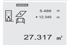
The painter's area function is used, for example, to determine the surface area of the walls in a room. This is done by determining the total length of all walls and multiplying this figure by the height of the room.
