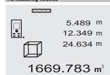
Each step of the volume measurement operation is indicated graphically in the display. For example, to determine the volume of a room, proceed as follows:
