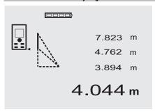
Follow the symbols in the display. The blinking side of the triangle indicates the measurement to be taken. When the 3 required distances have been measured, the result is then calculated and shown in the result line at the bottom of the display.
