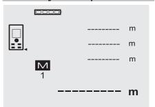
Data memory can be completely cleared by pressing the C-button for approx. 2 seconds while data memory is displayed.
