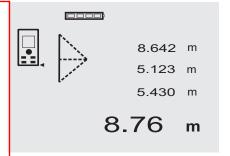
follow the symbols in the display. The blinking side of the triangle indicates the measurement to be taken. When the 3 required distances have been measured, the result is then calculated and shown in the result line at the bottom of the display.
