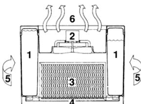
All evaporation occurs in the humidifier so any residue remains in the wick. This natural process of evaporation creates no white dust like some other humidifiers.
