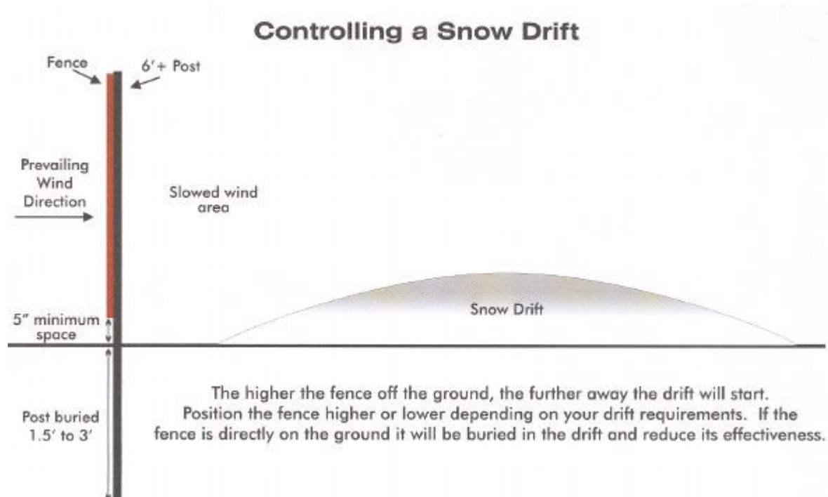
When snow blows and drifts on roadways or driveways, the end result often includes a reduction in driver safety, degradation of road quality, and significant removal costs for drifted snow. Snow fences are also used to trap snow in dugouts for water storage. The value of a snow fence is clear; however, exactly how one works is commonly misunderstood.
