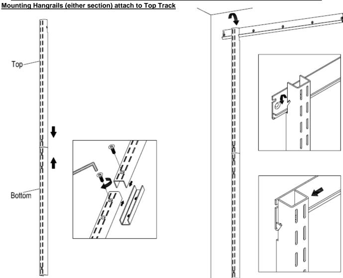
(above) assemble with hang rail slotted ends to outside Make sure notches are at the far end of assembled hang rail and space the hang rails on the Top Track 30-3/8" apart measured inside (between) the hang rails
