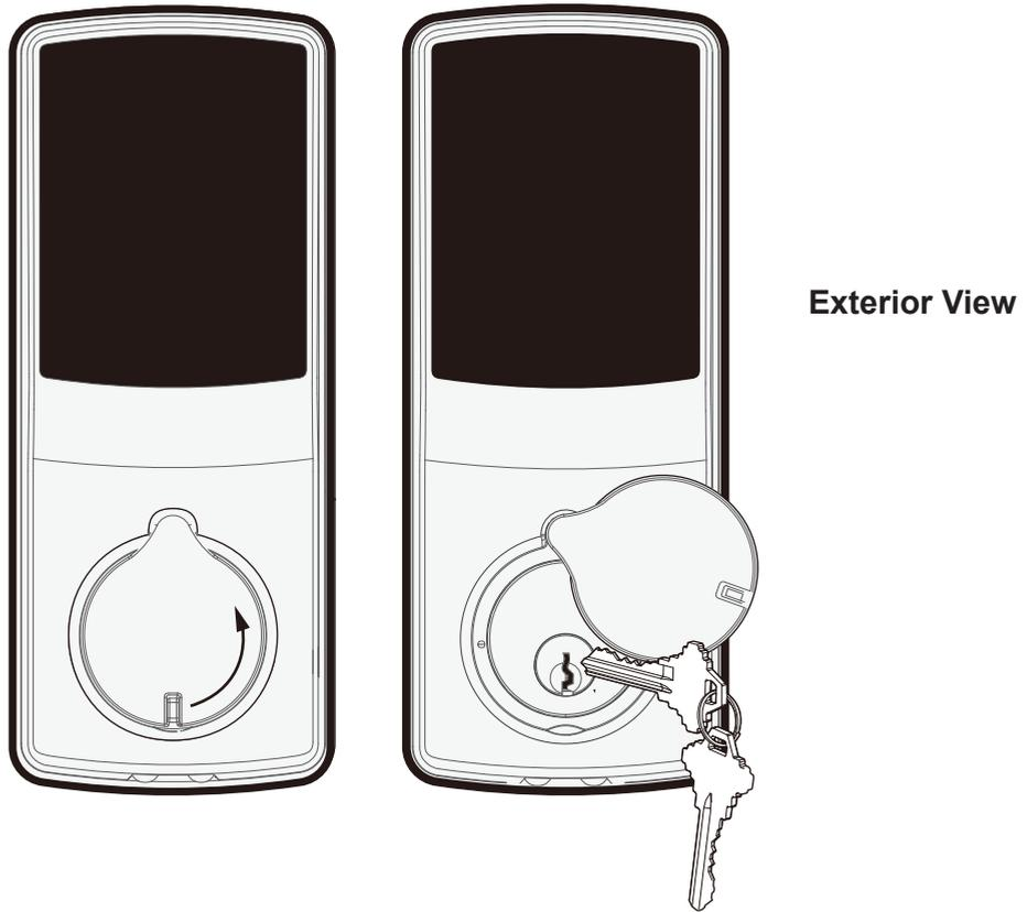
To **unlock** your Lockly™ using the **physical key (supplied)**, open the key cover on the handle by turning the cover counter clockwise to reveal the **keyhole**.
