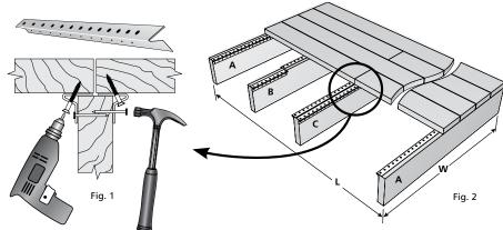
Installation Nail or screw hidden deck fasteners to the inside edges of outer joists (A), alternate edges of inner joists (B), and both edges of joists where decking is spliced (C), as shown above. Hammer nails in every other hole of the hidden deck fastener. Starting at one end of the joists, attach deck boards with two screws at each joist. (Fig. 1)
