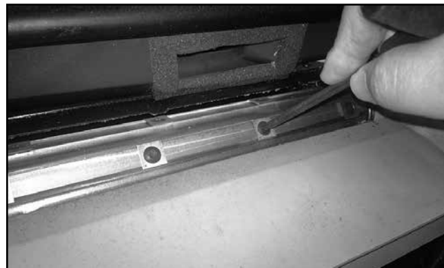
10. Place each insert in the housing and firmly secure it in place with a screw.
