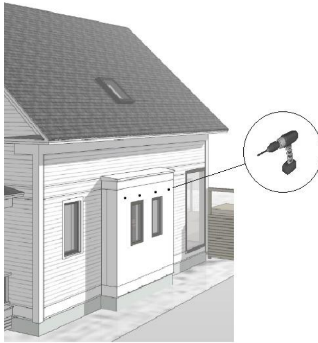
Figure G2: Installing (n) Shroud (Hood Cover) to the Pilot Holes
