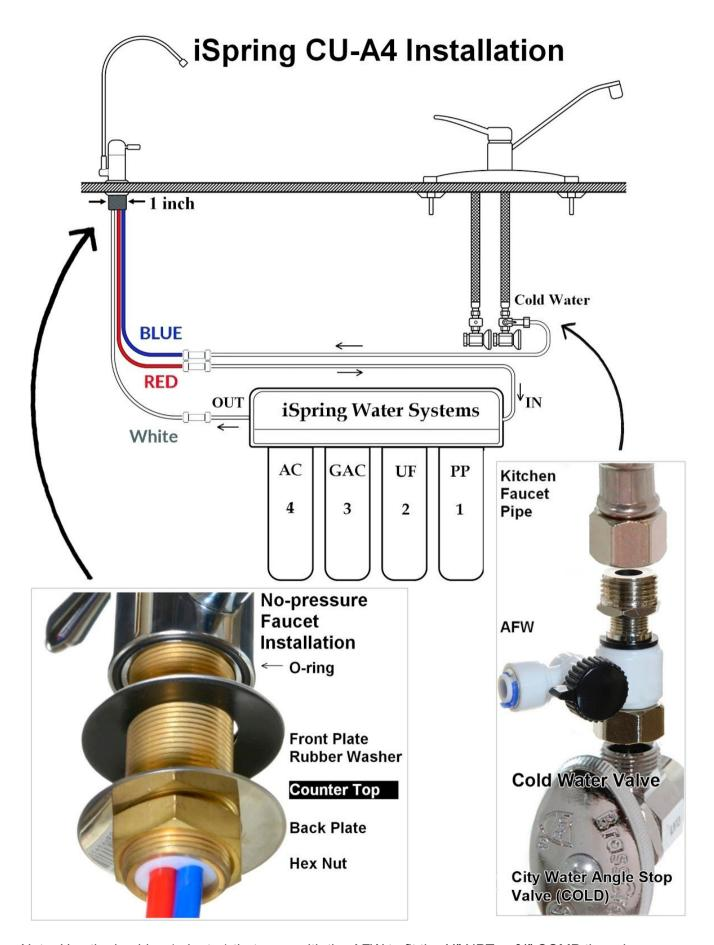
Note: Use the bushing (adapter) that goes with the AFW to fit the ½" NPT or ¾" COMP threads on your sink's Cold Water Pipe.
