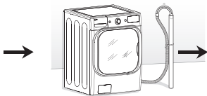
Connecting the drain line
