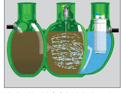
chamber hydraulic currents shall enter the sludge return and be directed through the Bio-Static device into the second zone of the clarification chamber. The Bio-Static sludge return shall accomplish resuspension and return of settled solids without disturbing the clarified liquid in the final settling zone and outlet zone.
