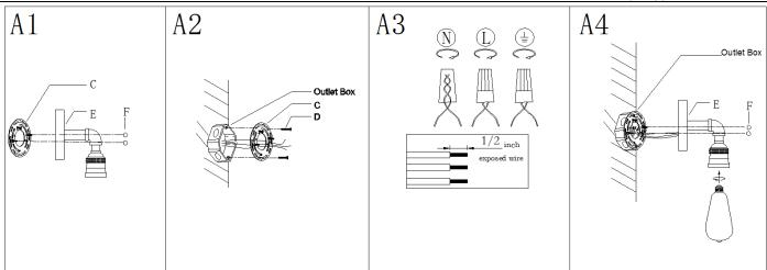
Step A1: Unscrew the knob nut(F) from back plate(E) then gently remove mounting plate (C)
