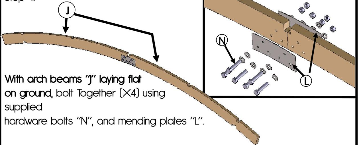
With arch beams "j" laying flat on ground, bolt Together (X4) using supplied hardware bolts "N", and mending plates "L".
