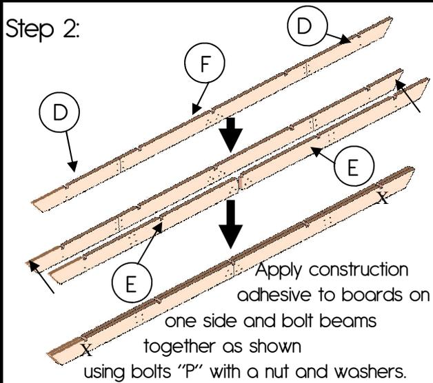
Apply construction adhesive to boards on one side and bolt beams together as shown using bolts "P" with a nut and washers. Bolt heads should be on the side comprised of beams "E" (Do not use bolts in holes marked with an X above.) Repeat for opposite side ledger beam. Insert 2" wood screws "S" into pre-drilled holes near ends of beams "D" once bolts are in place and tightened.
