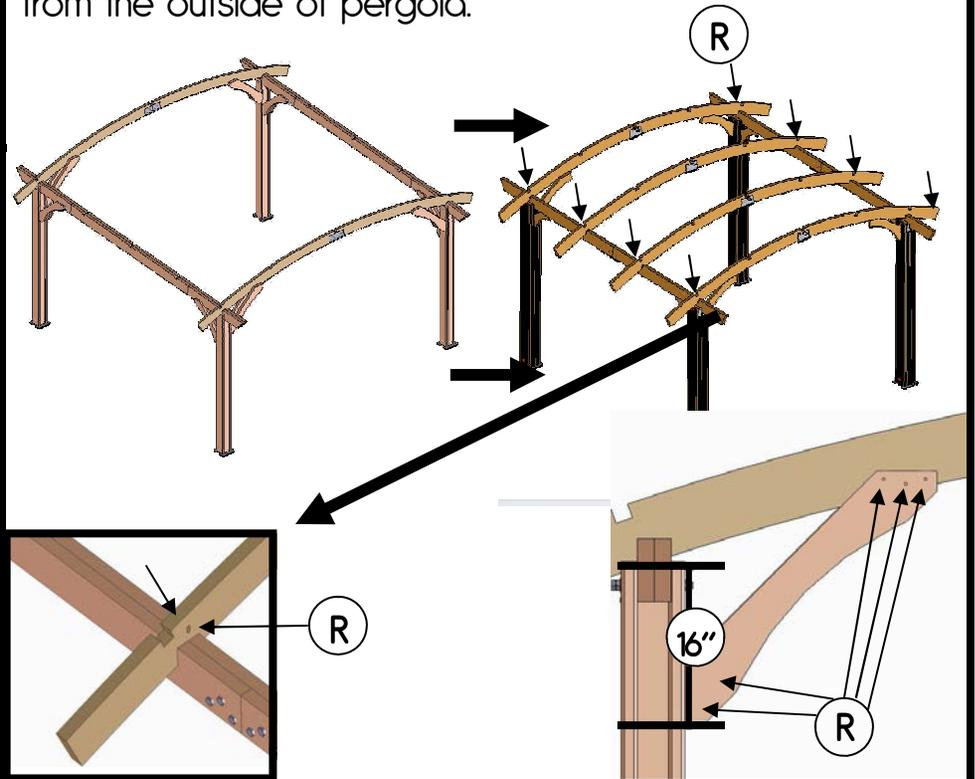
Insert 2 screws "R" into each side of column. Ensure columns are squared with ledger beam before fastening. Repeat for all columns.
