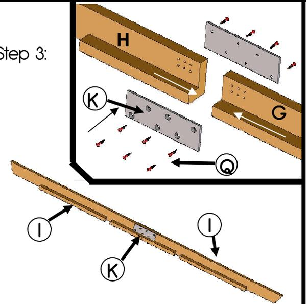
Attach rectangular mending plates "I" to canopy beams as shown. Attach beams "G" to beams "H" [x2], and beams "I" to "I" [x3]
