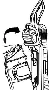
**Warning:** Do not touch the gears or switches located on the main body below the dust bin.
