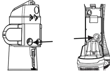
4. Check the hose where it connects body to head by turning the connector on the bottom of the body.
