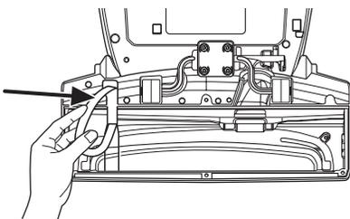
5. Fit the agitator through the belt, making sure the belt is aligned with the pulley section of the agitator.
