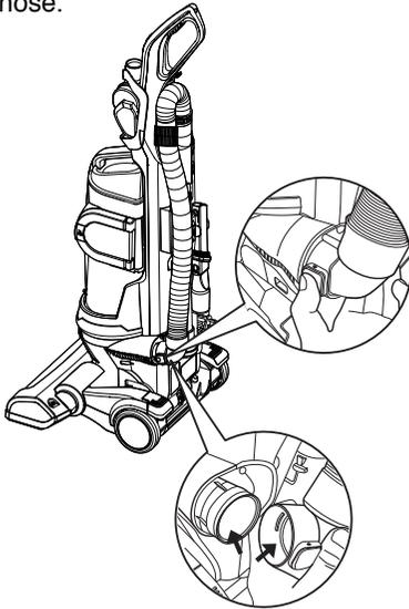
2. Release the hose assembly from the vacuum cleaner. Separate the hose and wand by pressing the button on the top of wand and check the hose and wand for clogs.
