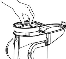
4. Separate the foam filter from the filter frame.
