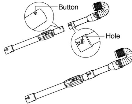
2. Attach the opposite side of the hose onto the main body.
