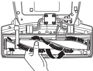
3. Unhook the old belt from the drive pulley. Make sure no pieces of the broken belt are trapped in the agitator or drive pulley area.
