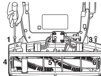
4. Carefully remove any accumulated string, hair, etc. from the agitator and the agitator area. To reinstall the cover. Reverse the steps above.
