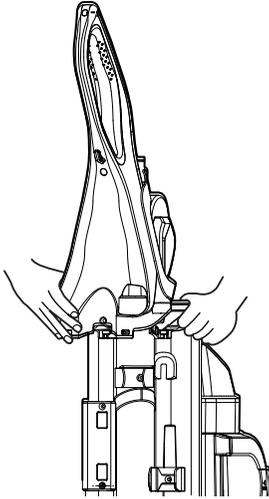
**Note:** Cord rewind button is in the up position when inserting into the main body. It is recommended to leave the tape on the button until the body and handle are assembled
