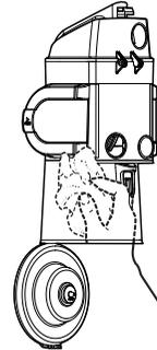
4. Release the latch on the Side door on both the right and left sides.
