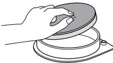
5. Shake out any excess dirt or debris and rinse the foam filter & filter frame with clean water.
