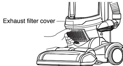
2. Lift out the filter by pressing the hook.
