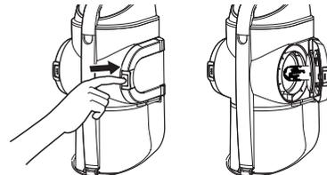
5. Remove any hair, fibers or other debris from the dust separator.
