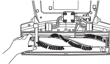
6. Lower the agitator into place, making sure the oval shaped tabs fit into the indents on the head.
