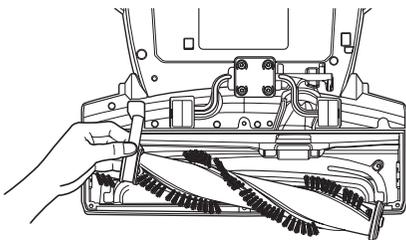
4. Hook the new belt over drive pulley of agitator motor.
