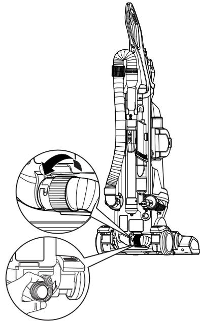
5. Turn the vacuum cleaner over, Check the agitator inlet.
