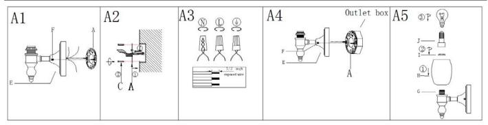
Step A1: Unscrew the knob nut(F) from back plate(E) then gently remove mounting plate (A)
