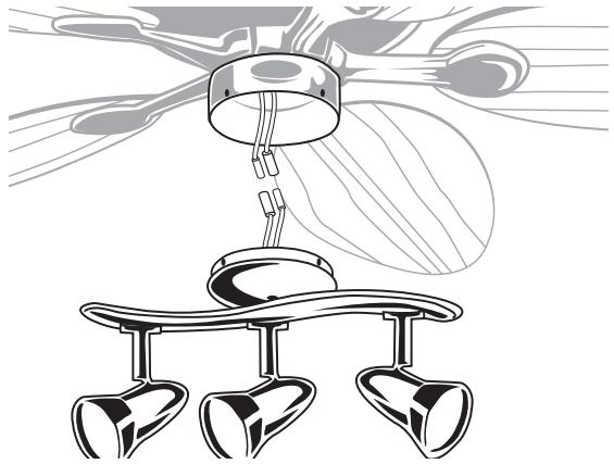
Attach light kit to the switch housing using three small screws provided.
