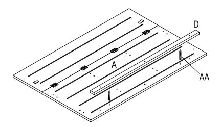
□ b) Tighten bar (D) with screw (EE).
