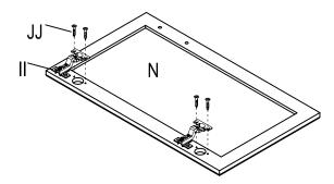
b) Attach left door (M) and right door (N) to the assembled body with screw (JJ) as shown.
