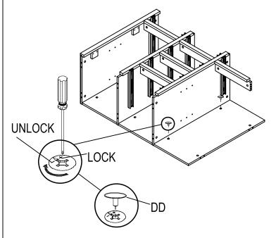
e) Cover the cam holes with the cover (DD).
