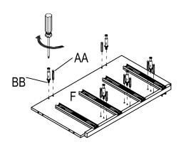
$\hfill\Box$   $\hfill$  c) Join panel (P) and bar (I) to the partition (F).
