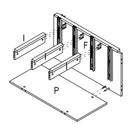
b) Insert lock (CC) into panel (P) and bar (I).
