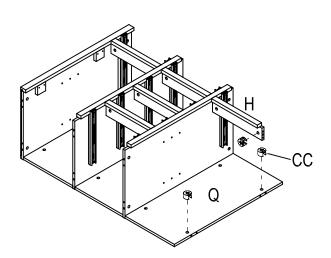
□ c) Join panel (C) to the assembled body with dowel (AA).
