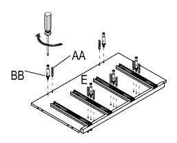
□ c) Join partition (E) to the assembled body with dowel (AA).
