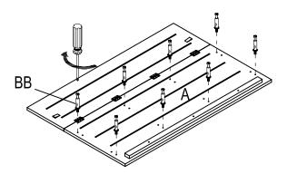
b) Insert lock (CC) and dowel (AA) into panels (B),(E), (F) and (C).
