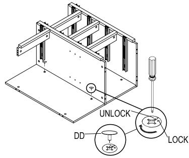
Wood dowel Cam lock bolt Cam lock Plastic cover Small head Large head
