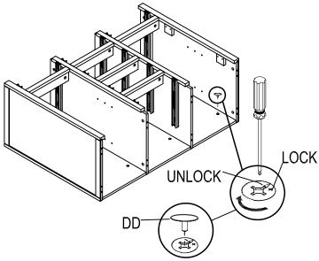
□ e) Cover the cam holes with the cover (DD).
