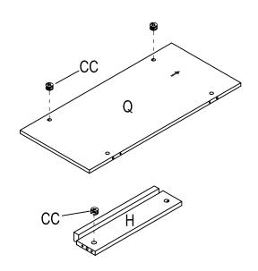
c) Join panel (Q) and bar (H) to the assembled body with dowel (AA).
