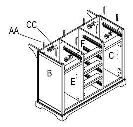
□ c) Join panel (A) to the assembled body with dowel (AA).
