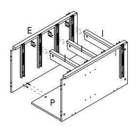
□ b) Insert lock (CC) into panel (P) and bar (I).
