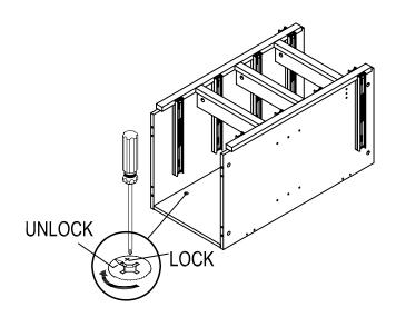
Wood dowel Cam lock bolt Cam lock Small head Large head
