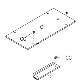
c) Join panel (0) and bar (G) to the assembled body with dowel (AA).
