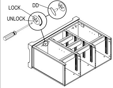
$\Box$  e) Cover the cam holes with the cover (DD).
