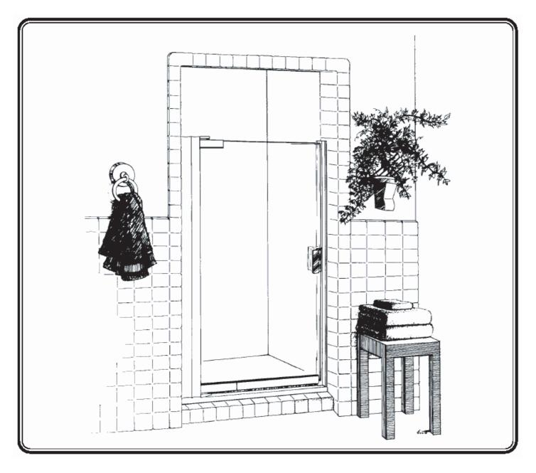
**MAINTENANCE:** Two primary materials are used to manufacture your new shower enclosure:tempered glass and anodized aluminum. To assure a long lasting finish on the enclosure, wipe it down with a towel after each use. Never use a scouring agent to clean the aluminum.
