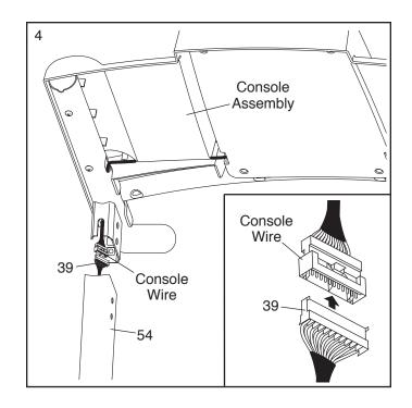
Set the console assembly on the Uprights (53, 54). Make sure that no wires are pinched.
