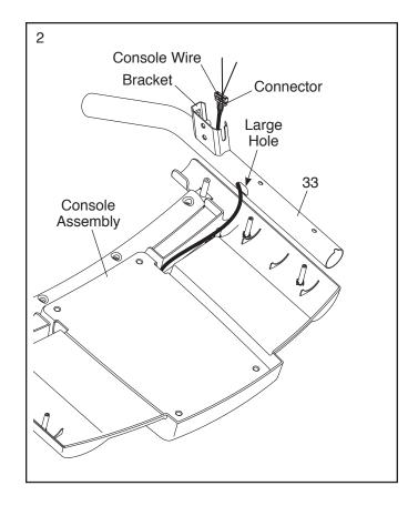
Set the Right Handrail (33) on the console assembly. Make sure that the console wire is not pinched. Remove the tie from the bracket on the Right Handrail. If necessary, press the Cage Nut (102) back into place.
