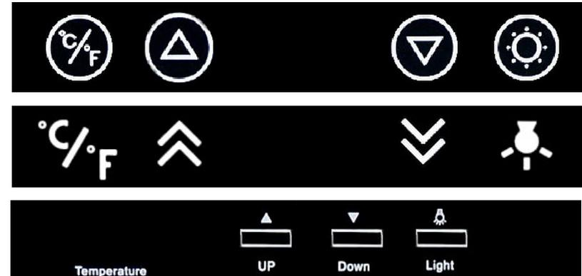
By pressing the (+) or (up arrow) temperature button on the display you can increase the temperature. Pressing the (-) (down arrow) temperature button will lower the temperature. Your wine cooler also has a light showcasing your wine and for added visibility. A light switch on the control panel will activate the LED light. Under normal operation it is best for the light to remain off.
